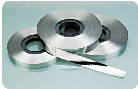
Nanocrystalline ribbon with 18 \mu m 1k107B (Fe-Cu-Nb-Si-B)
