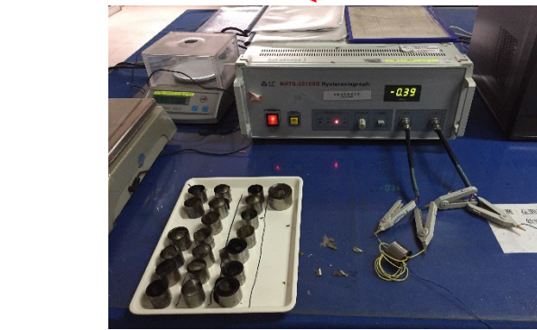
Testing the impact of the coating to the performance of small MA cores.
