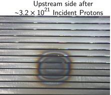
Reduce Material to Reduce Beam Loss
