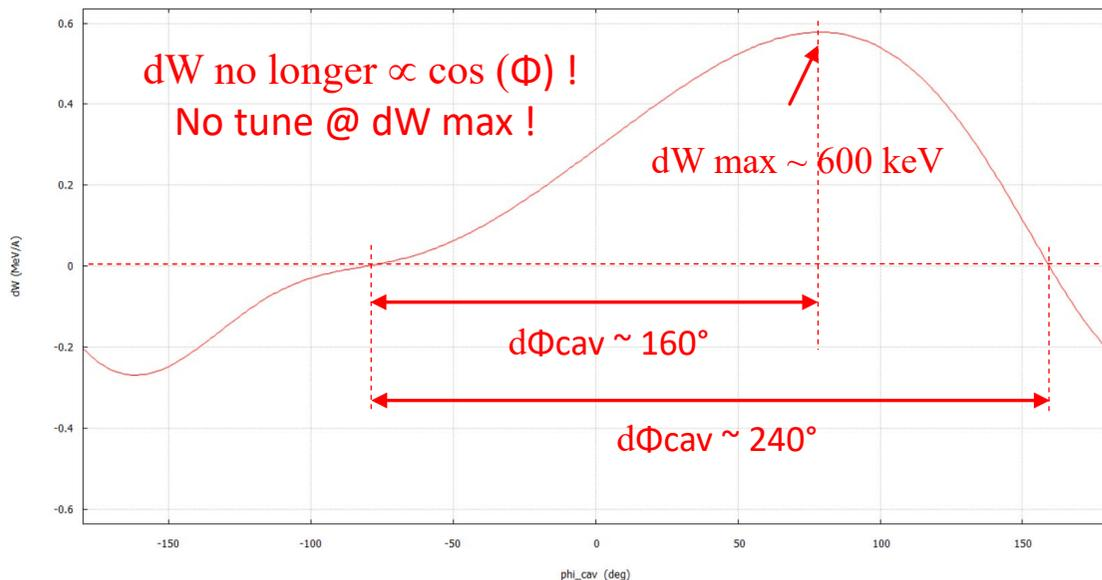
Energy gain for a  $-180 / +180^\circ$  cavity phase scan
