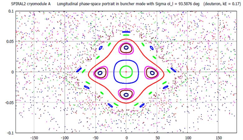
The  $\sigma_l = 90^\circ$  resonance main source of excitation (as well as the other parametric resonances in the longitudinal plane !)
