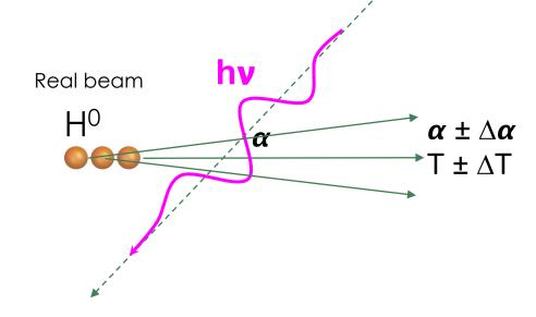
Most of the beam is not in resonant conditions
