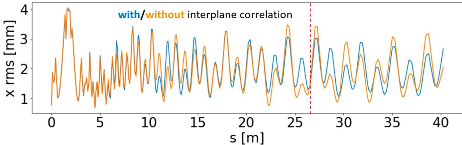
Figure 2: Comparison of horizontal beam size through PyORBIT simulation of SNS MEBT and DTL.
