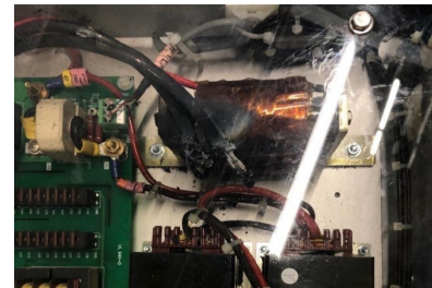
Defect transformer in microwave amplifier No more support New solid state version
