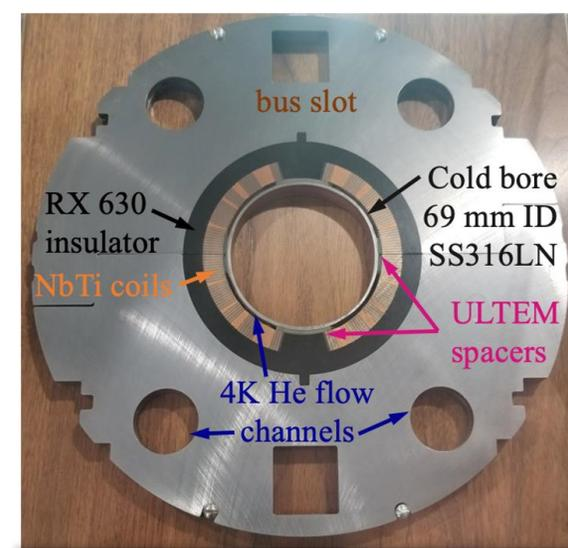
RHIC arc dipole cross section
