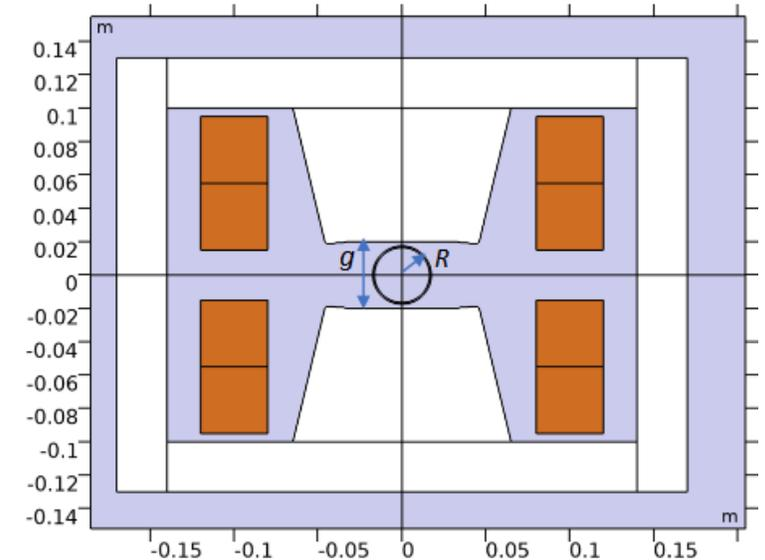
RCS vacuum chamber: Copper tube,  $R = 17.5 \text{ mm}$ ,  $t = 1 \text{ mm}$ .
