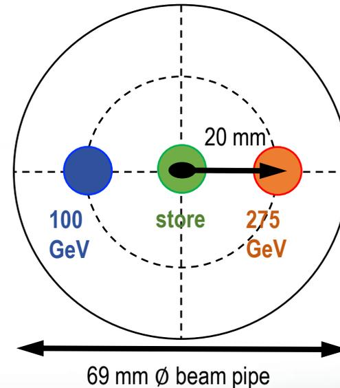
Large radial orbit offsets for collision beams in arc magnets
