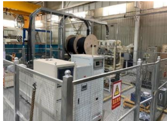
Kicker power supply test with real load
