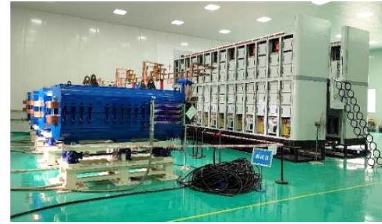
Field measurement of bending magnets
