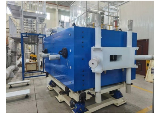
Superferric bending magnet with warm iron
