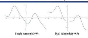
Reduce the longitudinal peak current intensity, and thus reduce the beam loss caused by space charge effect.
