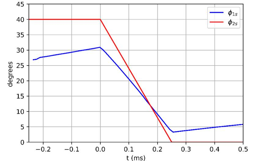
A combination of  $r=0.8$  and momentum offset of  $-0.15\%$  was used, that is, the longitudinal emittance after injection was 1.78 eVs. Second harmonic phase sweep was used during injection
