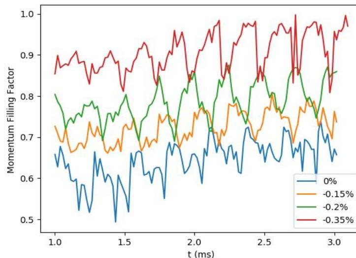
Since the upgrade project of 200kW **doesn't include the momentum collimator at the first place**, the momentum spread should be **controlled under 1%** to avoid that large beam loss occur in arc section, and **the corresponding momentum filling factor is 0.8**.
