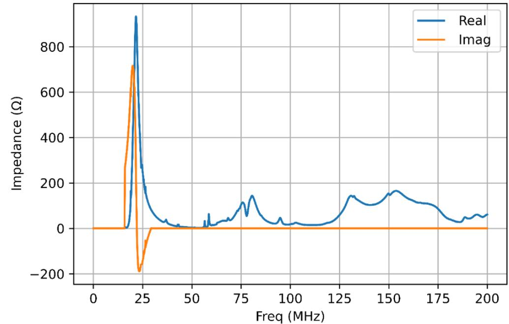
longitudinal impedance of MA Cavity
