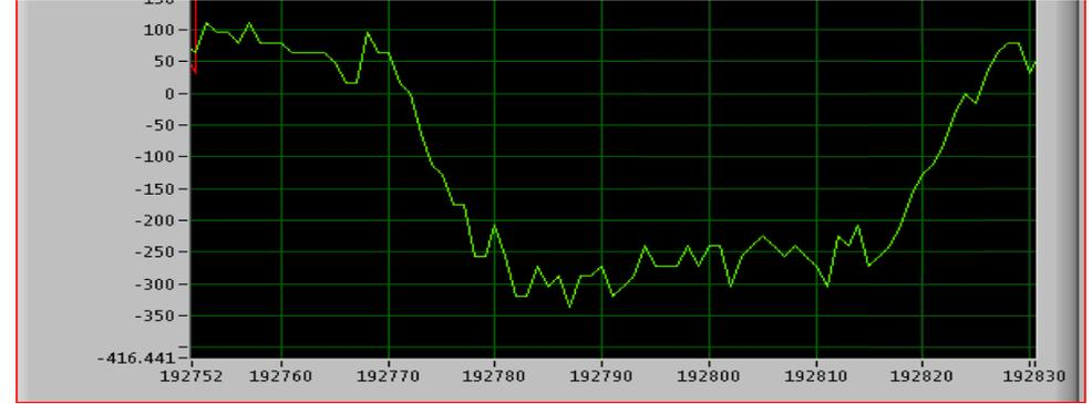
Add magnetic alloy cavity,  $r=0.8$ , adjust the second harmonic phase, ensure the peak height of both sides same(phase calibration)
