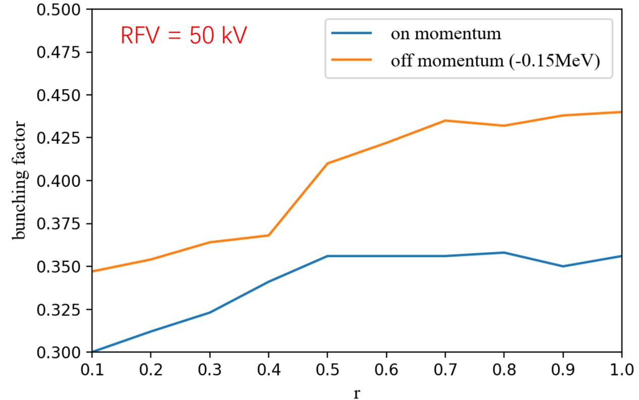
**Combining injection momentum offset with a large second harmonic cavity voltage can better increase the bunching factor.**
