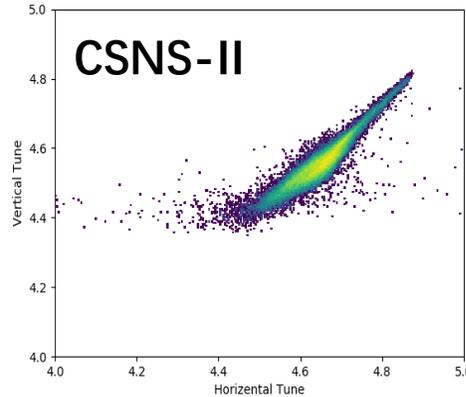
The tune spread at 500 kW is much smaller than at 100 kW.
