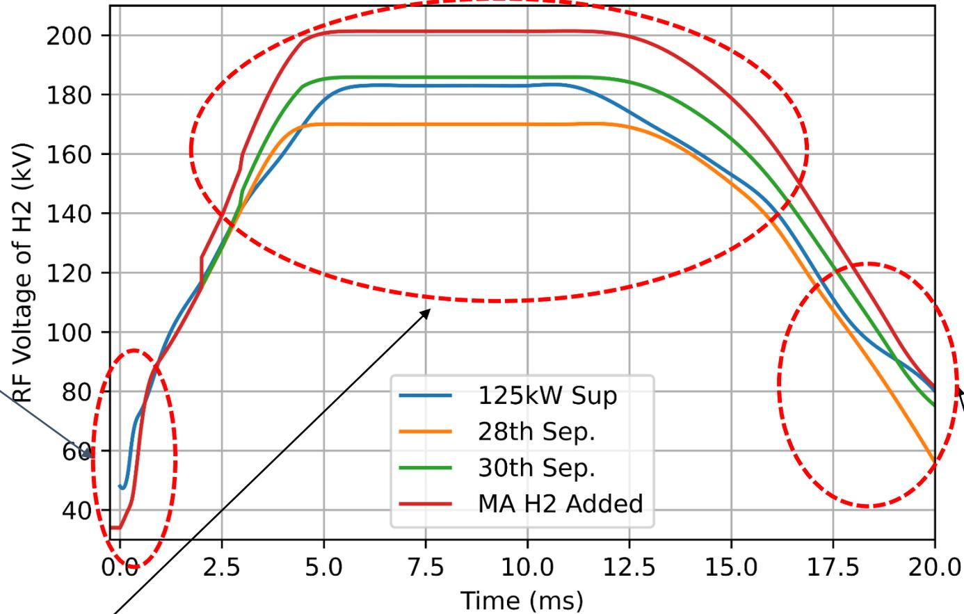
Matching of synchronous oscillation period and injection turn. Also increase the voltage ratio equivalently.
