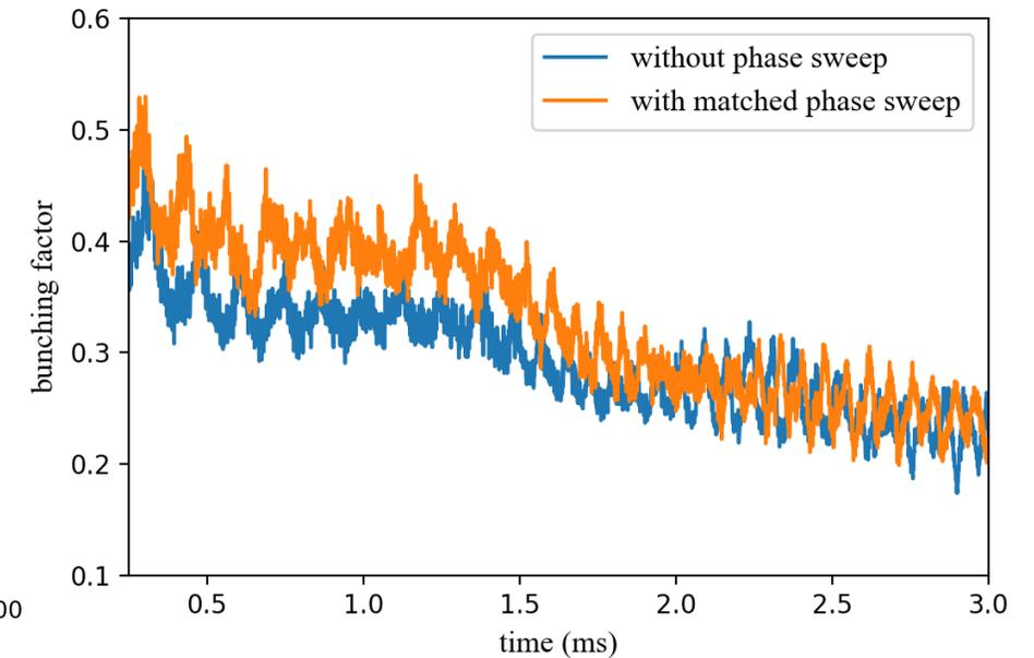
Bunching factor is higher with a matched phase sweep method. Additionally, the beam loss can also increase by approximately 3% with this method.
