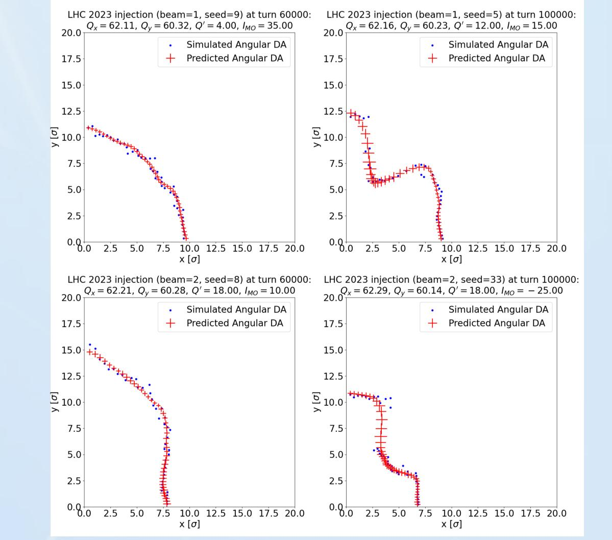
Mean Absolute Error (MAE) used as loss function. Inference in 1  $\mu$ s/angular DA (0.5 ms/ machine configuration). **MAE = 0.201 beam**  $\sigma$  in test dataset. Mean Absolute Percentage Error (MAPE) = 11.91%.
