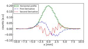
Figure 9: Normalised horizontal beam profile after the ABS septum magnet (about 8 m downstream of the splitter).
