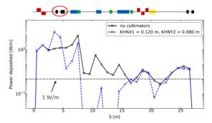
Figure 7: Power deposition from splitter to target with optimal collimator settings. Collimator positions are circled in red. 1 W/m level is marked with an arrow.
