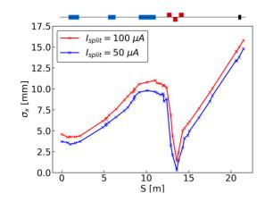
Figure 4: Horizontal beam size of split beam along the TATTOOS beamline for 100 µA (red) and 50 µA (blue) split beam currents.
