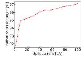
Figure 5: Transmission of split beam from splitter to TATTOOS target for different split beam currents.
