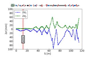
Figure 6: Beam sizes from extraction to SINQ target. Splitter location is marked with dashed red lines.
