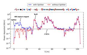
Figure 8: Power deposition from the extraction of the Ring cyclotron to SINQ target. Case with splitter in the beamline and operating at 100  $\mu$ A (blue curve) is compared to case without splitter (red curve).
