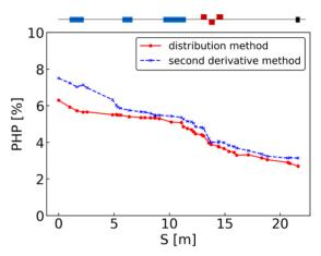
Figure 10: Evolution of the beam halo along the TATTOOS beamline for 100  $\mu$ A split beam current using two different methods.
