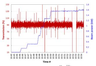
Figure 5: Power ramp up of  $80 \mu A^{40} Ar^{14+}$  beam: Transmission (red) and beam power (blue).
