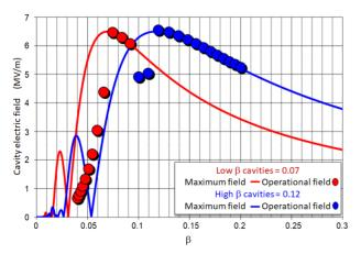
Figure 2: SPIRAL2 Transit Time Factor for: the maximal (line) and the operational (points) electric fields.
