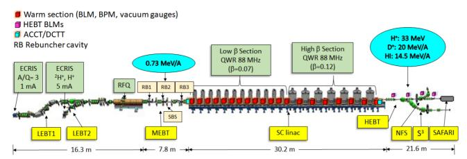
Figure 1: SPIRAL2 SC linac layout
