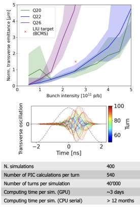
Figure 5: Simulation study for the CERN SPS based on simulations including the full non-linear lattice, space charge (PIC model) and wakefields. Top: obtained instability thresholds for different beam optics; middle: one of the simulated instabilities; bottom: some relevant simulation parameters.
