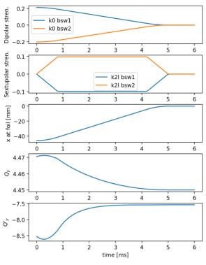
Figure 1: Simulation of a fast orbit bump used for the H<sup>-</sup> injection into the CERN PS Booster. From top to bottom: 1) Time dependence of the dipolar strength of two of the dipole correctors; 2) corresponding sextupolar components from induced eddy currents; 3) resulting position at the stripping foil as computed by Xsuite; 4) effect of the dipole change on the vertical tune (mostly due to fringe fields); 5) effect of the dipole change on the vertical chromaticity.
