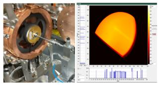
Figure 4: Left: single-slice graphite target inside the watercooled copper enclosure. Right: thermal image of a 10 kW, 216.7 MeV/u  $^{48}$ Ca beam on the target rotating at 500 revolutions per minute.
