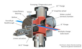
Figure 3: Intermediate-power charge selector design (1'' = 25.4 mm).
