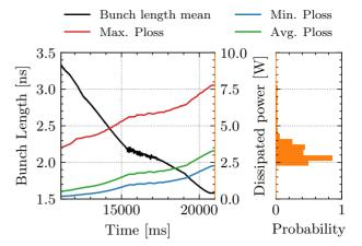
Figure 6: Power loss evolution in time during the ramp (second y-axis). The bunch length evolution in time is reported on the first y-axis. A histogram reporting the probability of having a certain dissipated power value, for the last time step of the computation, is shown on the right side. The number of protons per bunch is the LIU target intensity of  $N_b = 2.3 \cdot 10^{11}$ . The filling pattern consists of 4 trains of 72 bunches with 25 ns spacing (SPS standard).
