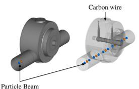
Figure 5: 3D CAD model of the SPS beam wire scanners.
