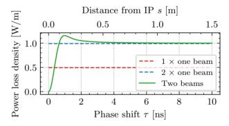
Figure 3: Power loss distribution along one half of the CBP. The behaviour is symmetrical in the other half of the pipe.
