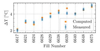
Figure 4: Thermal excursion measured by the probe located at 50 mm from the IP and the simulated thermal excursion.
