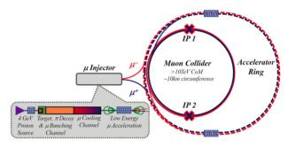
Figure 1: Proposed layout of a muon collider and its muon production and acceleration stages. Picture from Ref. [6].
