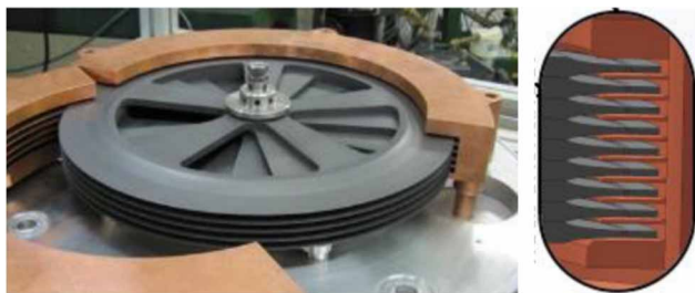
Figure 4: Left: Multi-slice graphite target with part of the cooling jacket out of copper. Right: Sketch showing the stacked targets at the rim [21].
