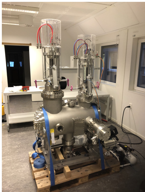
Figure 2: The two LEBT FC in the tank for testing prior to installation in the ESS linac.
